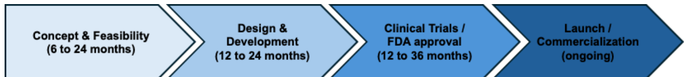
Figure 3 High-level product development process for medical devices
