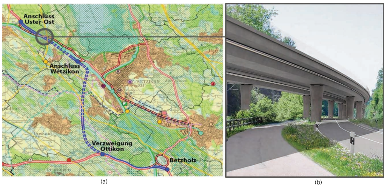
Figure 1. (a) Diagram of planned completion of the A15 highway (Kanton Zürich, 2019) with the tunnels marked with a dashed blue line, the open street sections with a continuous blue line and position of the new bridge in Aathal marked with a grey circle ('Anschluss' means 'junction', and 'Verzweigung' means 'branching'); (b) a render of the planned bridge in Aathal (Redaktion Züriost, 2020)
